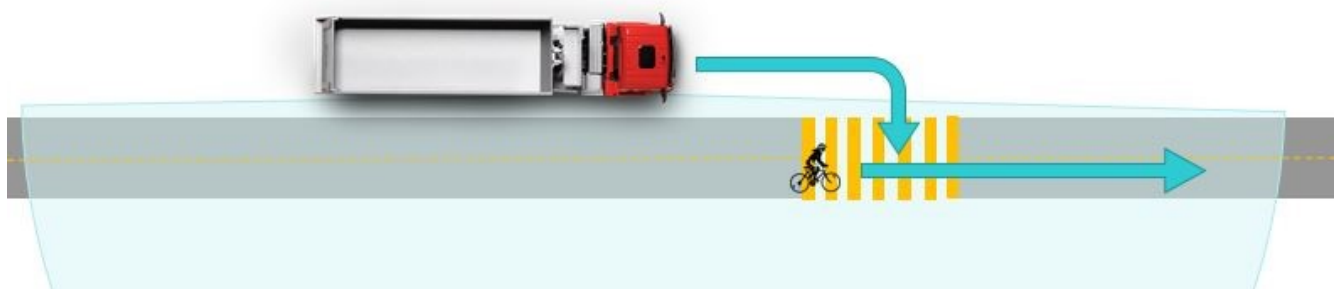
Figure 1 - Example scenario: Vehicle at 20 km/h with bicycle at 10 km/h in front of the vehicle
