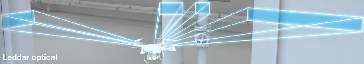
Multi-segment Leddar optical sensors provide vital object/surface detection and positioning over a wide field-of-view, indoor or outdoor.
