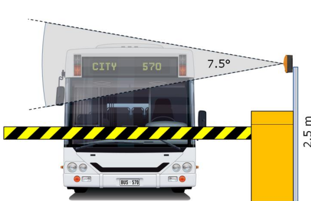
Fig. 1: 45° sensor opens the barrier gate upon detection of buses only (front view)
