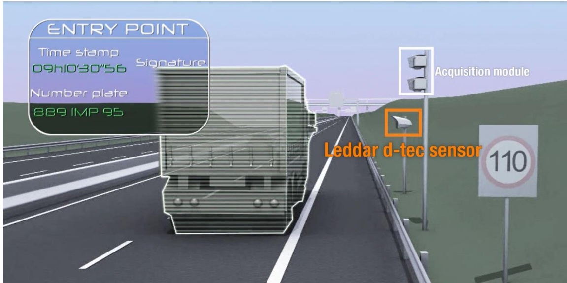
Conceptualization of the Mesta 5000 automated average speed control system at entry point. Source: Safran (Morpho). Image modified by LeddarTech.
