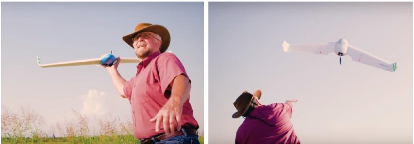
Figure 2 – Hand-launched take-off is performed by the operator by simply throwing the Eclipse drone in the air
