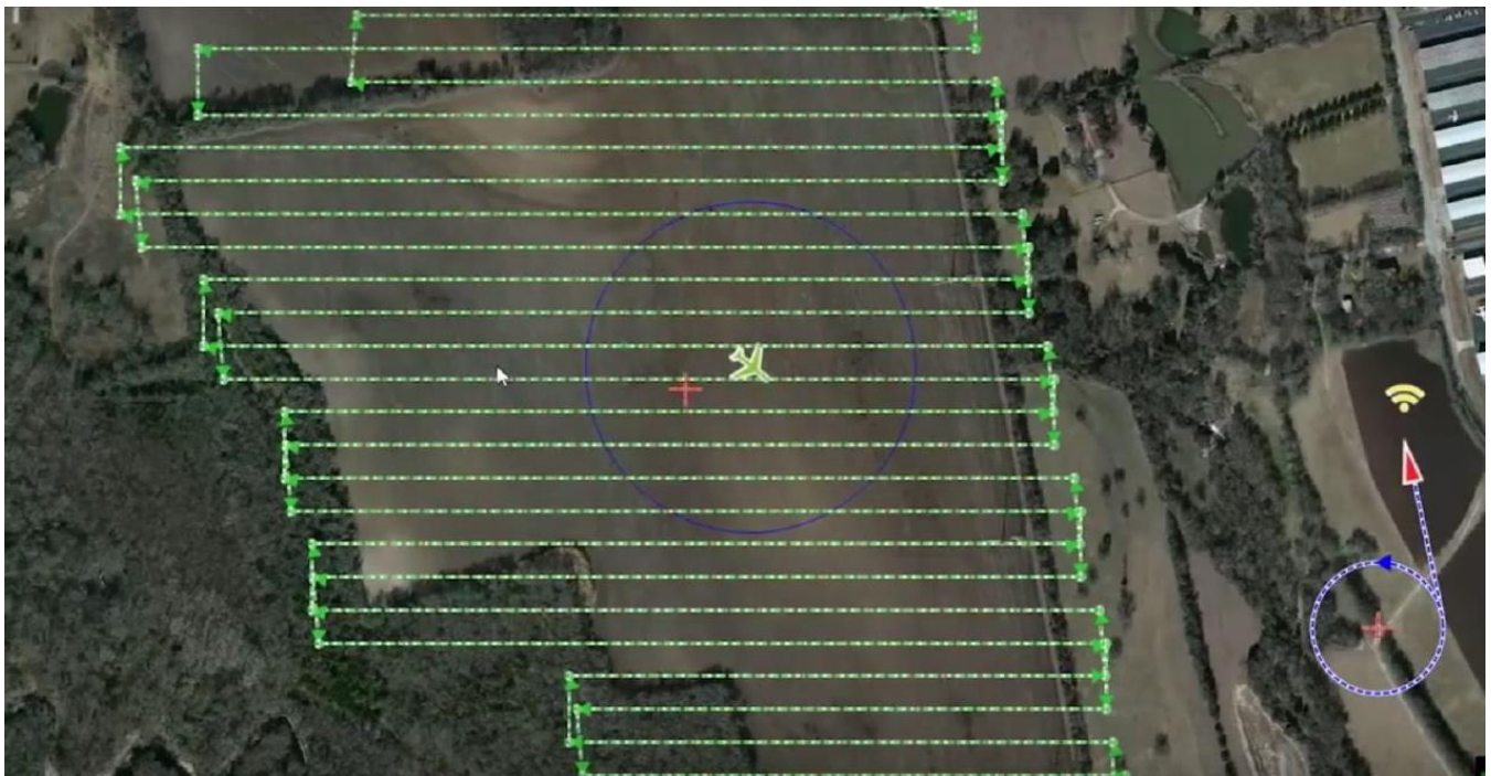
Figure 1 – Surveying drones follow a pre-set flight plan to capture data over a specific area before returning to the landing point
