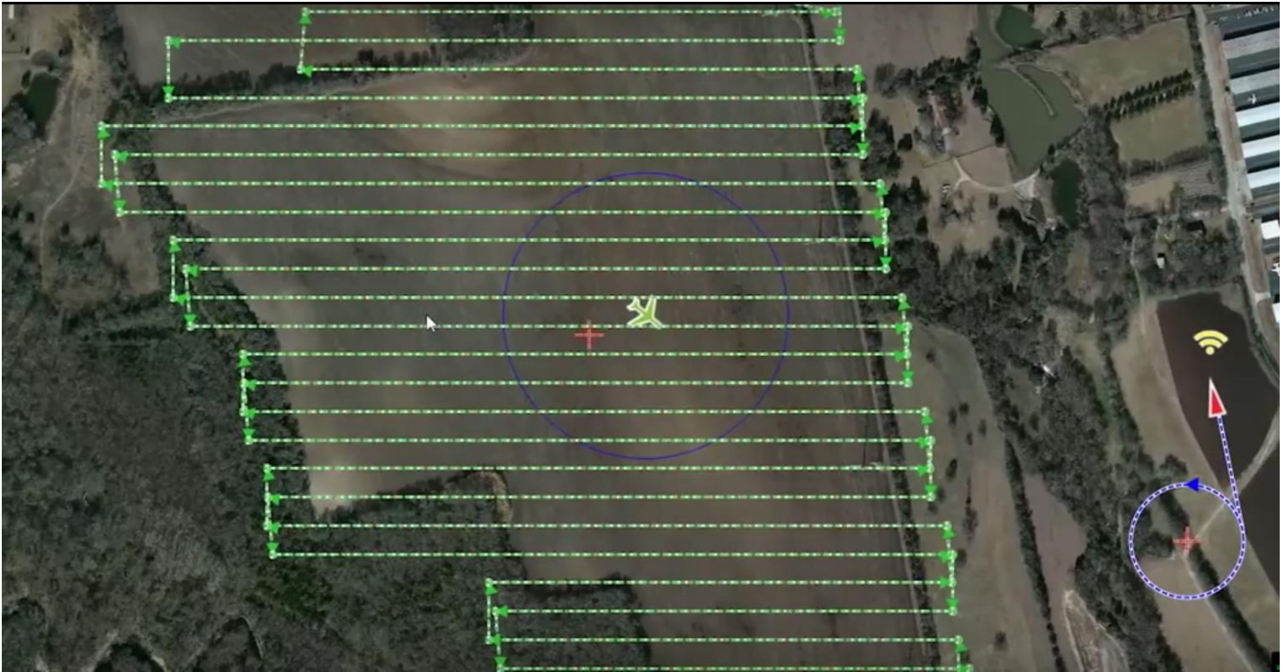
Surveying drones follow a pre-set flight plan to capture data over a specific area before returning to the landing point
