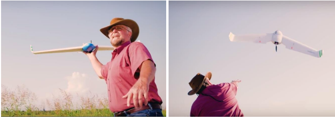
Hand-launched takeoff is performed by the operator by simply throwing the Eclipse drone in the air
