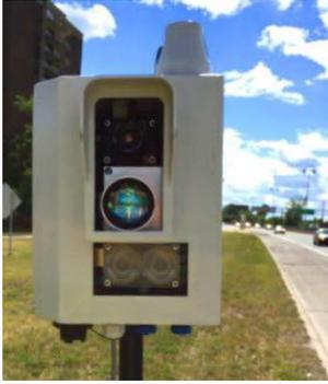
**Figure 1 – Enforcer Speed Camera System by LogixITS**
