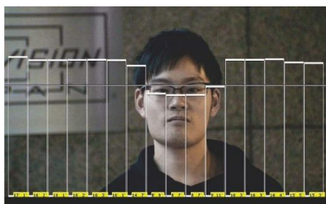
The subject distances are represented by an array of rectangles, each one representing one of the 16 detection zones of the Leddar M16 module
