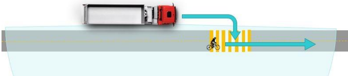
Figure 1 – Example scenario: vehicle at 20 km/h with bicycle at 10 km/h in front of the vehicle
