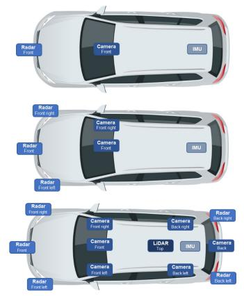
Figure 30 – Examples of sensor architecture, from basic to advanced
