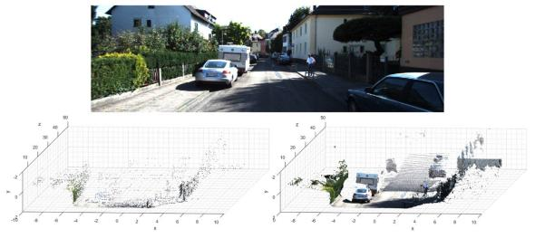
Figure 4 – 3D reconstruction example
