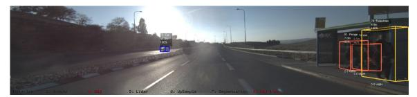
Figure 25 - Cars (on the left) and pedestrians (on the right) detected with blinding sun above
