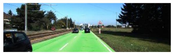
Figure 14 – Example of free-space detection (light green)
