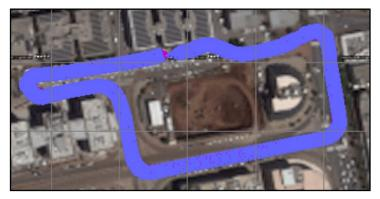
Figure 11 – Basic localization from a bird's-eye view (blue = ego-motion, pink = GNSS as ground truth)
