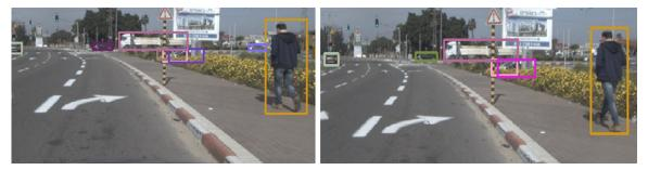
Figure 17 – ID switch on one distant and one occluded vehicle (left: distant = purple, occluded = blue. Right: distant = green, occluded = pink)
