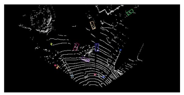
Figure 6 – 3D detection and enhancement (bird's-eye view based on LiDAR data)
