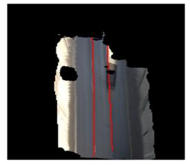
Figure 19 – Bird's-eye-view projection with a polynomial fit of the driving lane
