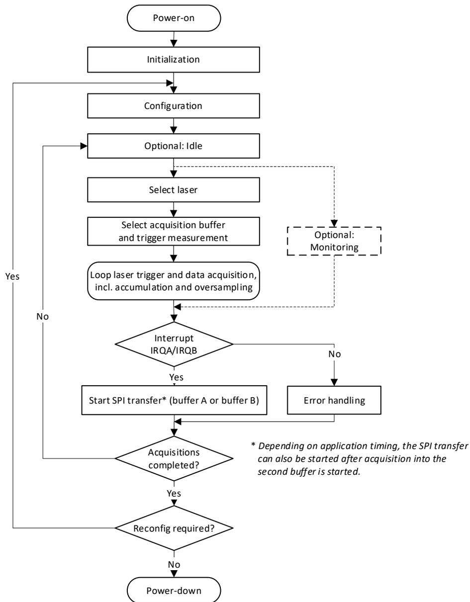
Figure 1 – Typical LiDAR application flow chart for LCA2 LeddarCore
