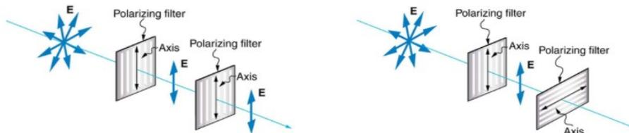
Figure 1 – Unpolarized light passing through filters set up in parallel and in perpendicular, respectively. Source: Lumenlearning.com
