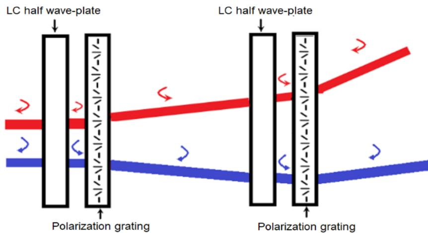
**Figure 3 – Two layers of liquid crystals used for beam steering**
