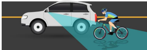
Figure 2 – Blind spot detection and intervention system
