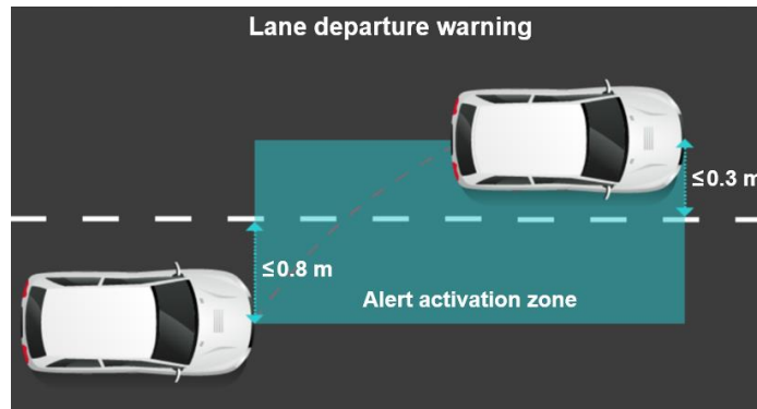
Figure 4 – Existing lane departure warning alert activation criteria
