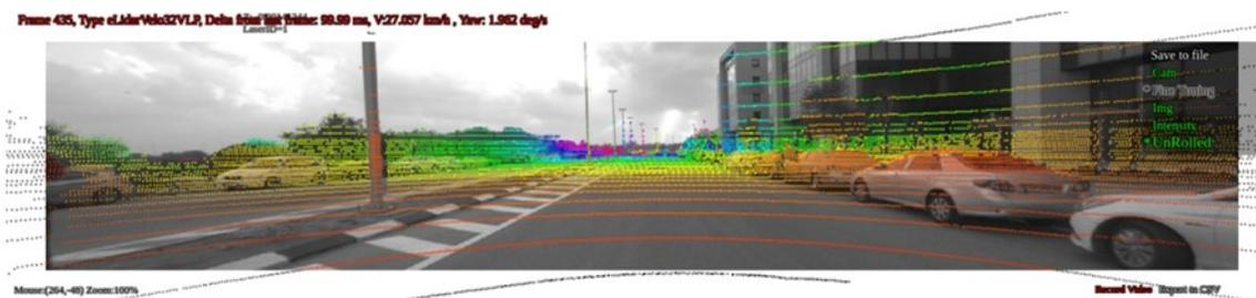
Figure 28 – Example of calibration between LiDAR point cloud and camera image
