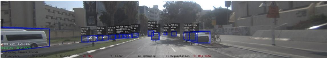
Figure 27 – Good detections in area of light transition (bright to shade on the right)
