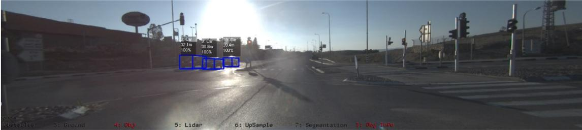
Figure 24 – Cars (on the left) detected with blinding sun above
