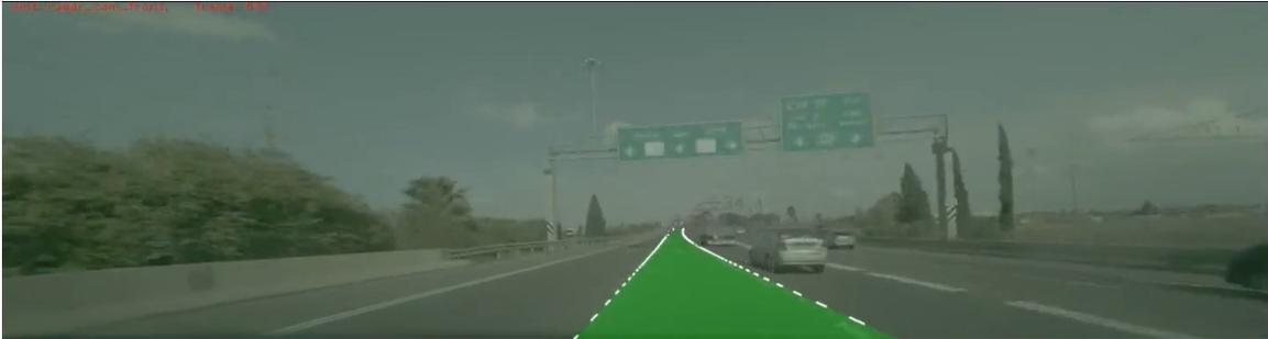
Figure 18 – Example of road and lane detection
