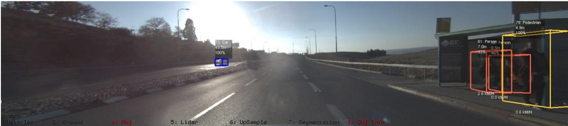
Figure 25 – Cars (on the left) and pedestrians (on the right) detected with blinding sun above
