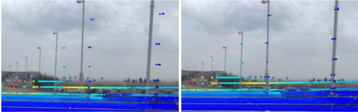
Figure 29 – Camera + LiDAR before calibration (left) and after calibration (right)
