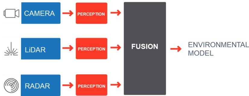
Figure 2 – Object-level fusion
