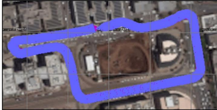
Figure 11 – Basic localization from a bird’s-eye view (blue = ego-motion, pink = GNSS as ground truth)
