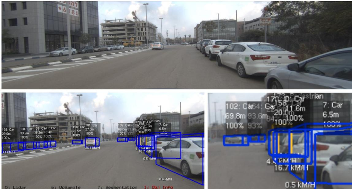
Figure 23 – Top: original image, showing partially occluded pedestrian detection.
