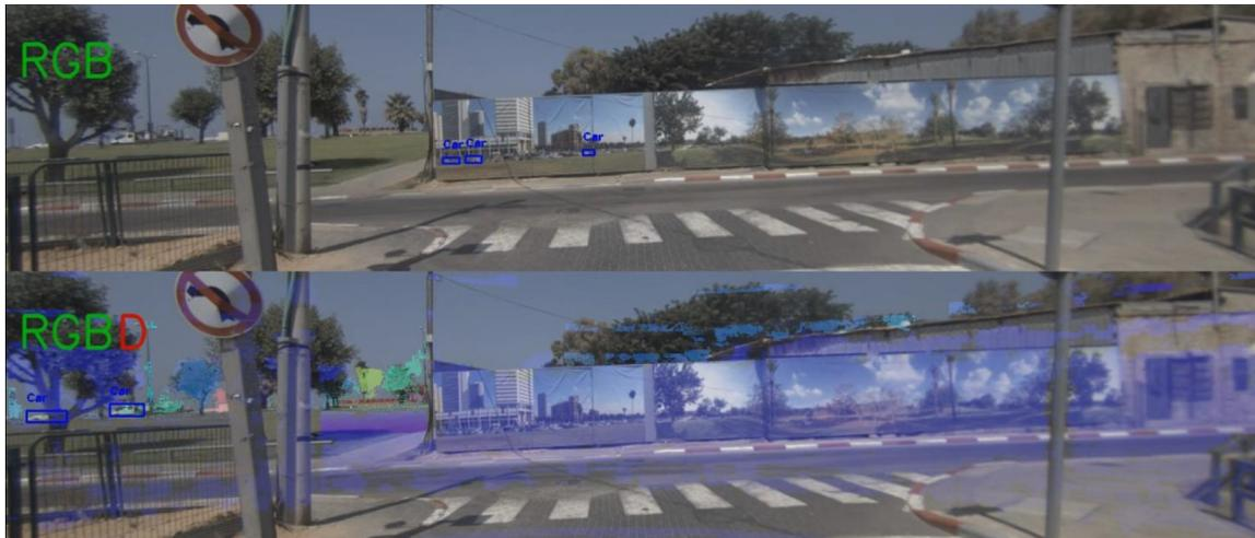
Figure 22 – Top: cars with no depth are detected (RGB detection).
