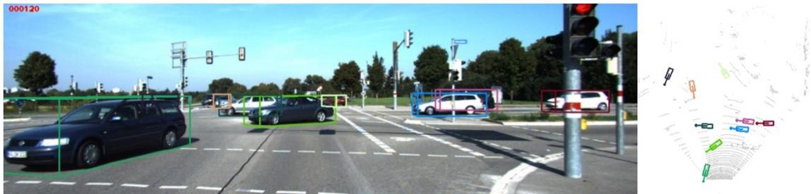
Figure 10 – Sample object trajectories (3D + bird's-eye view)
