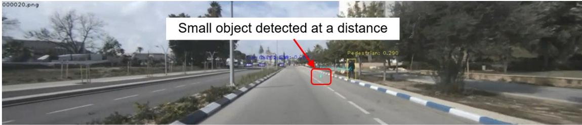
Figure 8 – Small-object detection, example 2 (object is detected at a distance)
