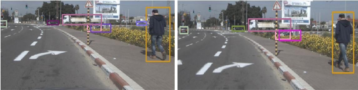
Figure 17 – ID switch on one distant and one occluded vehicle (left: distant = purple, occluded = blue. Right: distant = green, occluded = pink)
