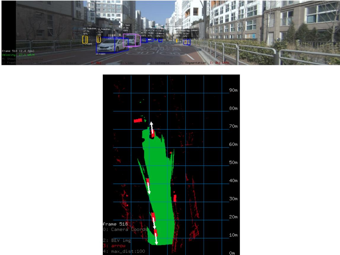
Figure 21 – Front view with detections (top) and corresponding occupancy grid (bottom)
