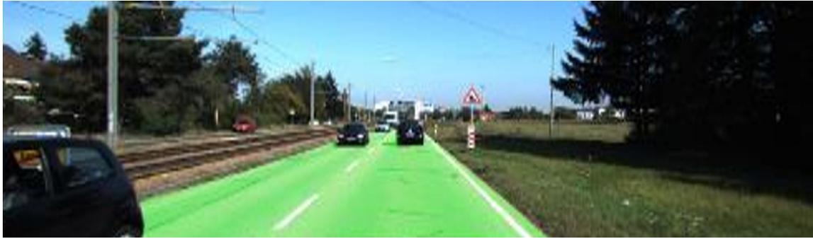
Figure 14 – Example of free-space detection (light green)
