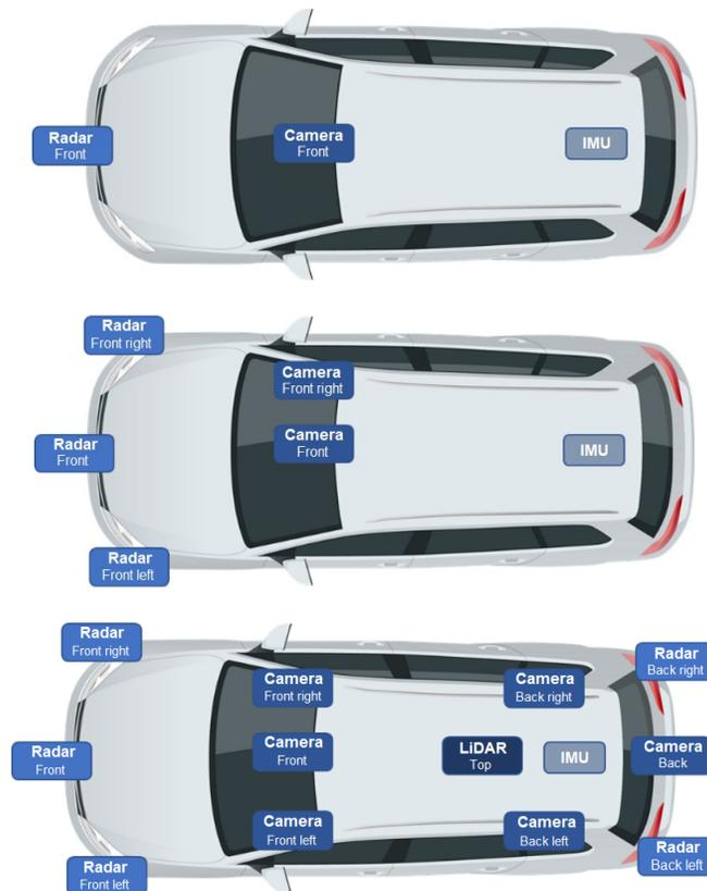
Figure 30 – Examples of sensor architecture, from basic to advanced
