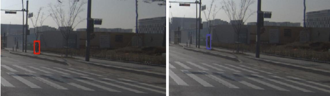
Figure 16 – ID switch on an occluded pedestrian (left: ID No. 1 = red; right: ID No. 2 = purple)
