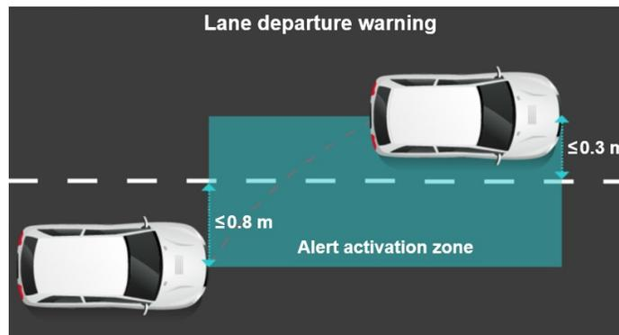
**Figure 4 – Existing lane departure warning alert activation criteria**
