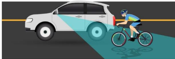
Figure 2 – Blind spot detection and intervention system
