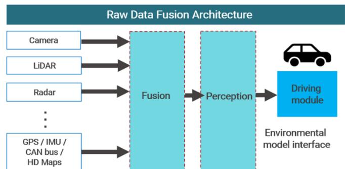
Raw data from sensors is first fused together. Detection and classification algorithms then run on the fused model. Decision is based on all sensors' input.
