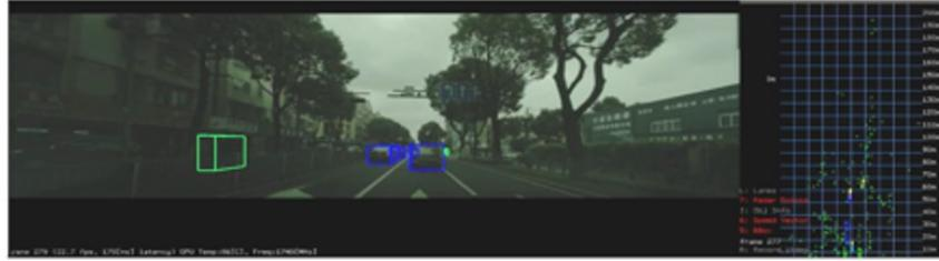
LiDAR/camera fusion (LCF)
