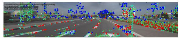
Figure 12 – Ego-motion keypoints (red = with depth, blue = without)
