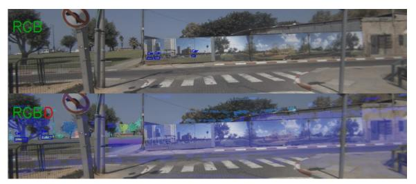
Figure 22 – Top: cars with no depth are detected (RGB detection). Bottom: only "real" cars are detected (RGBD detection).
