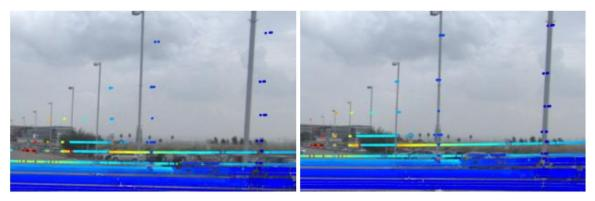
Figure 29 – Camera + LiDAR before calibration (left) and after calibration (right)
