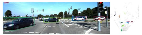
Figure 10 – Sample object trajectories (3D + bird's-eye view)
