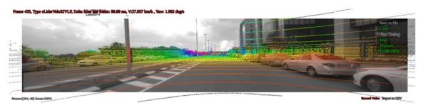
Figure 28 – Example of calibration between LiDAR point cloud and camera image
