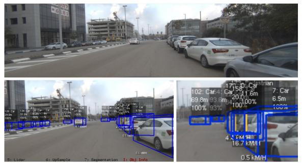
Figure 23 – Top: original image, showing partially occluded pedestrian detection. Bottom left: pedestrian (in yellow) is detected between two cars; bottom right: zoom-in of the scene.
